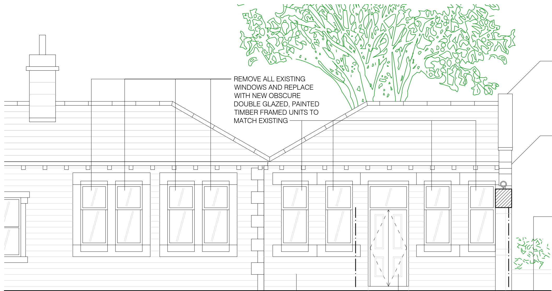
Proposed Side Elevation - CC Scale 1:50
