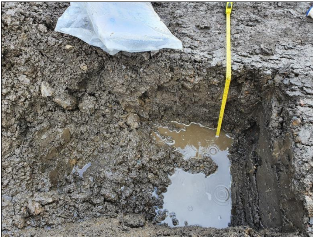
Plot 8 and 9: Validation trial pit showing depth to bottom.
