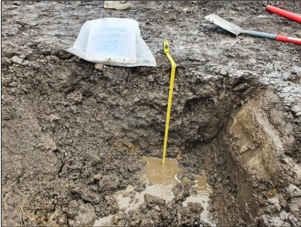
Plot 6 and 7: Validation trial pit showing depth to bottom.
