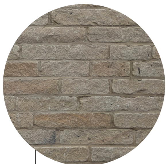
90MM COURSE NATURAL STONE GENERAL WALLING FROM JOHNSON WELLFIELD QUARRIES OR HILL HOUSE EDGE QUARRY
