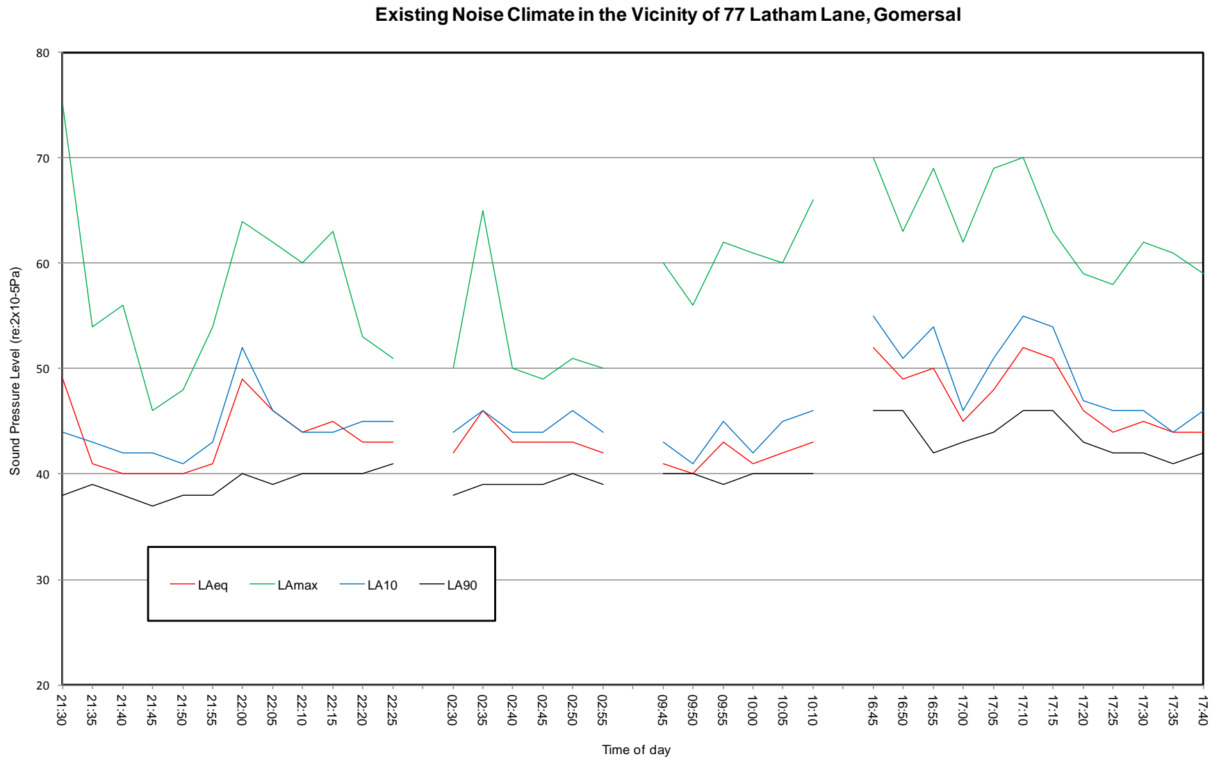
Graph 1. Existing noise climate measured noise levels, in the vicinity of 77 Lathom Lane, Gomersal
