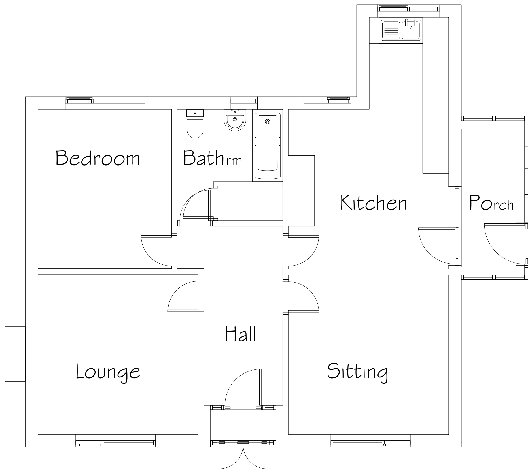
Existing Bungalow Floor Plan
