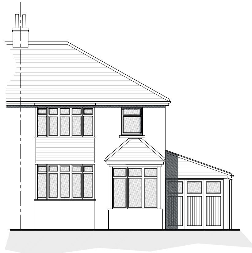
Existing North East Facing Front Elevation Scale 1:100
