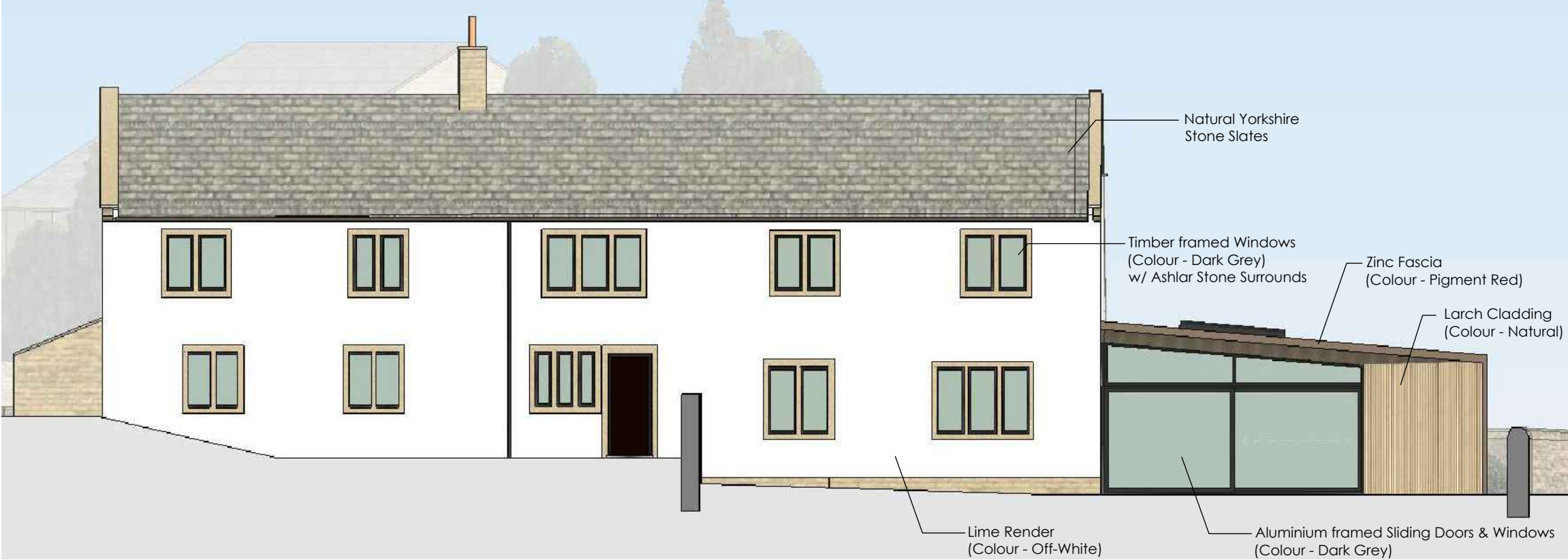
SOUTH WEST ELEVATION
