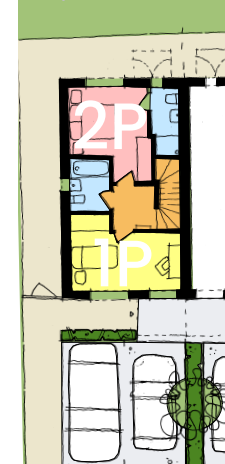
Typical 2B3P NDSS compliant house
