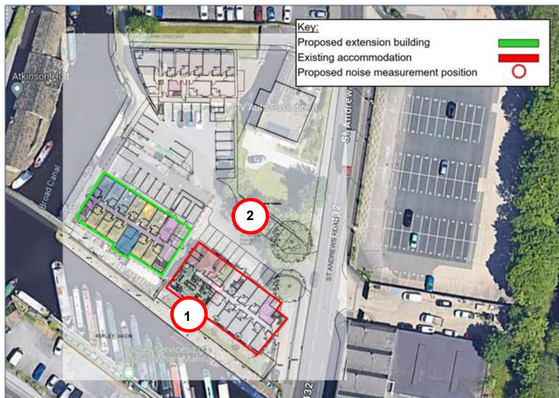
Figure 2.1: Site and noise measurement positions.
