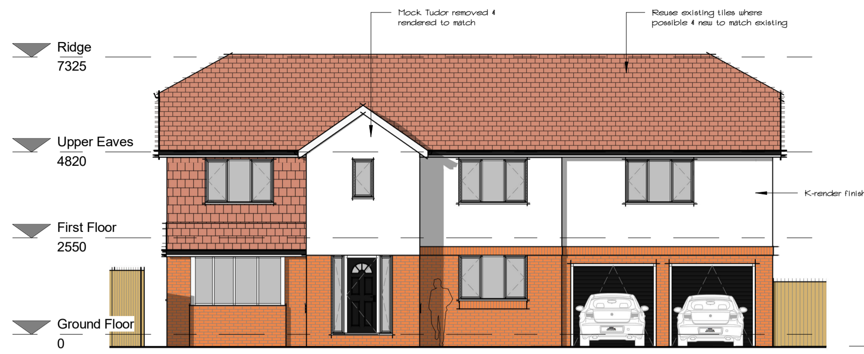
Front Elevation (SE Facing) 1: 100
