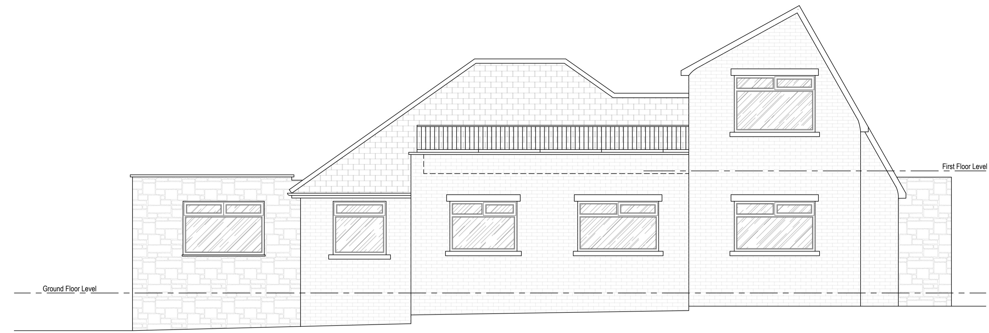
Existing Rear Elevation - East Scale 1/50
