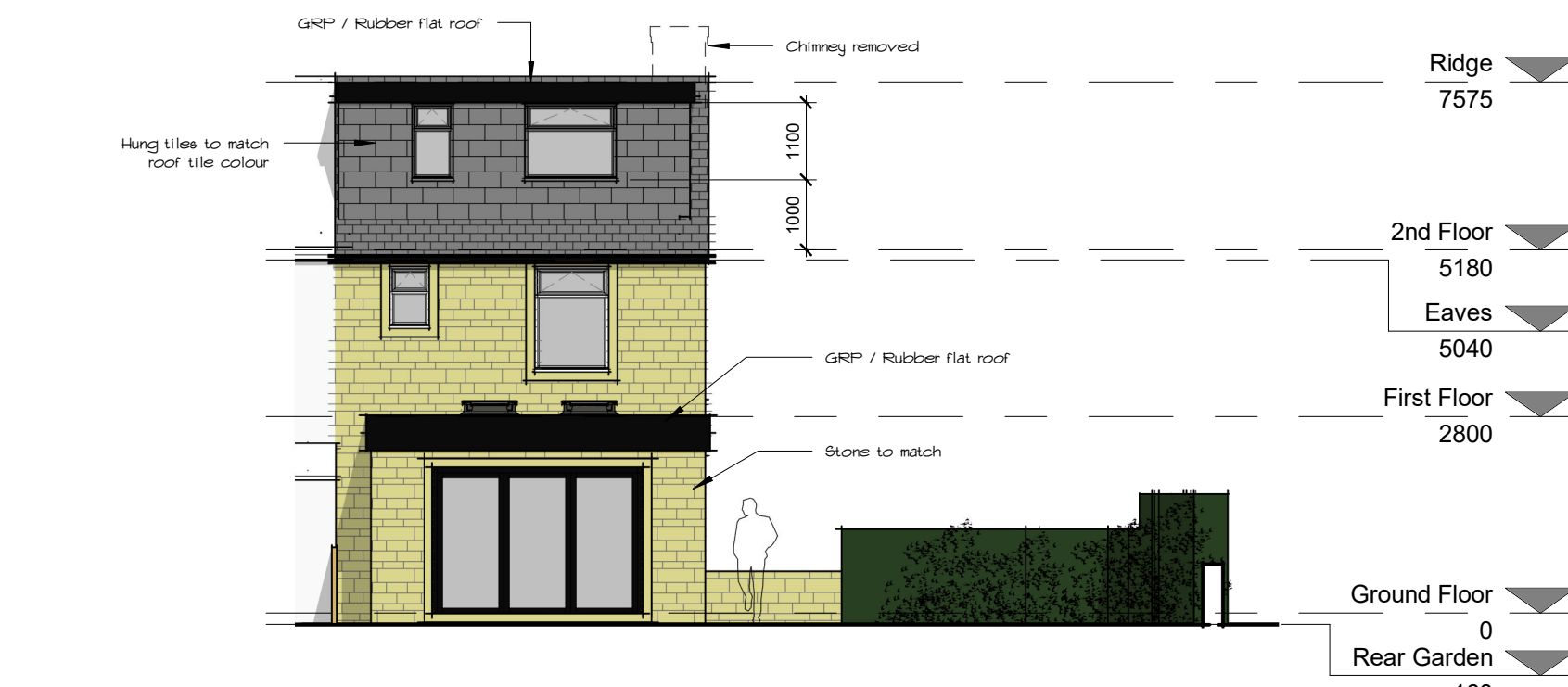
Rear Elevation (SW Facing) 1 : 100
