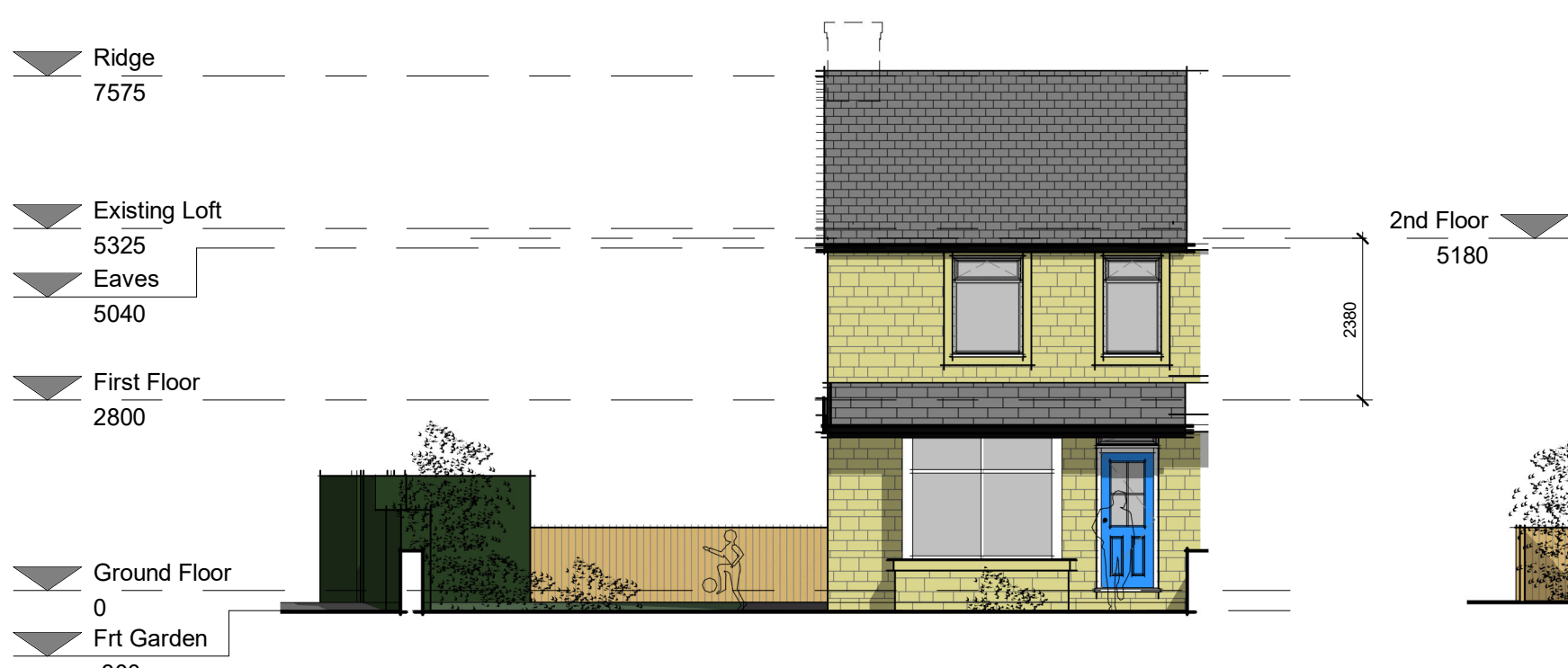
Front Elevation (NE Facing) 1 : 100
