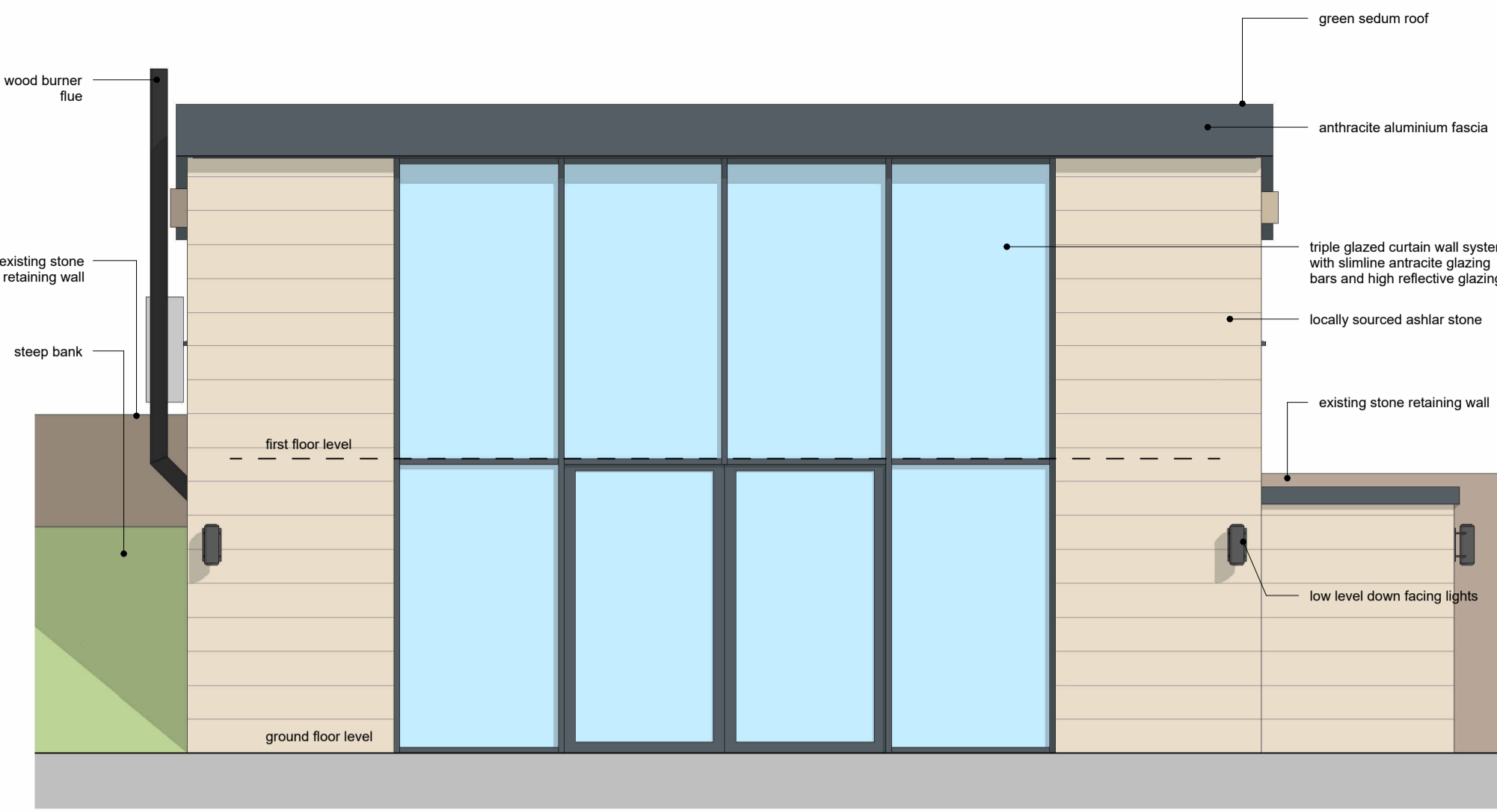
south east elevation (front) 1 : 50
