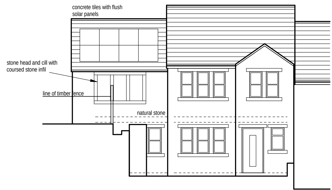
Proposed front elevation (1:100)
