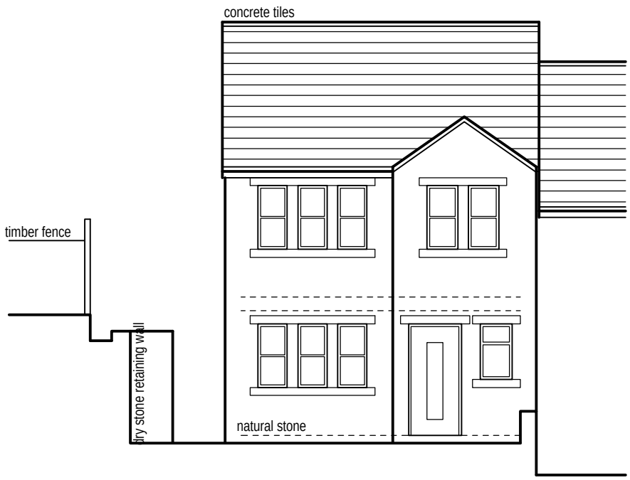
Existing front elevation (1:100)
