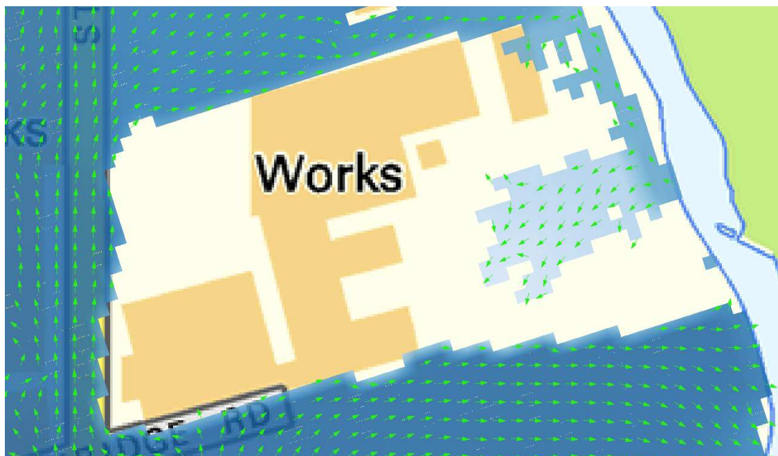
Figure 6.4: Initiation of on-site flooding for the 1 in 500 AP plus 20% event (flow direction in green arrows).
