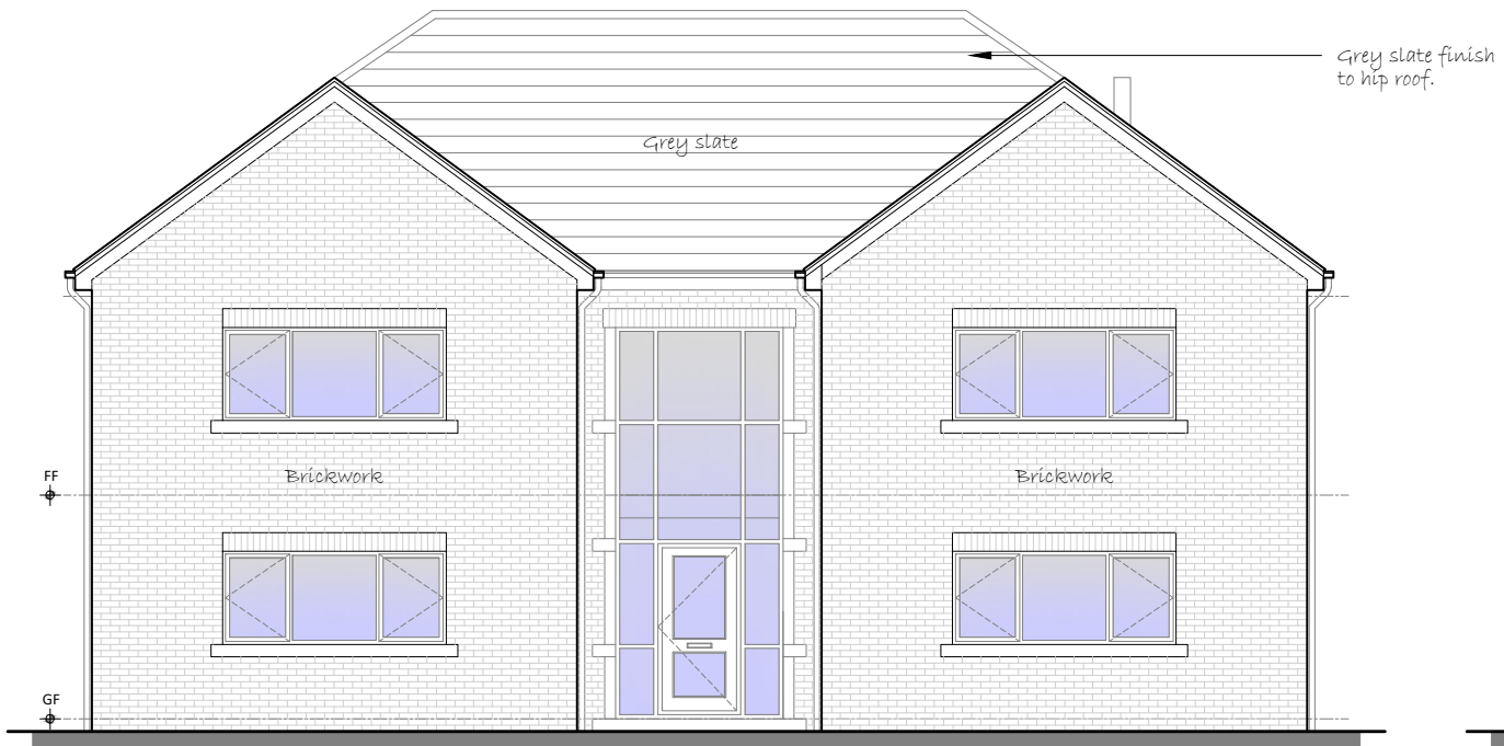
PROPOSED SOUTH-WEST (FRONT) ELEVATION SCALE - 1:100
