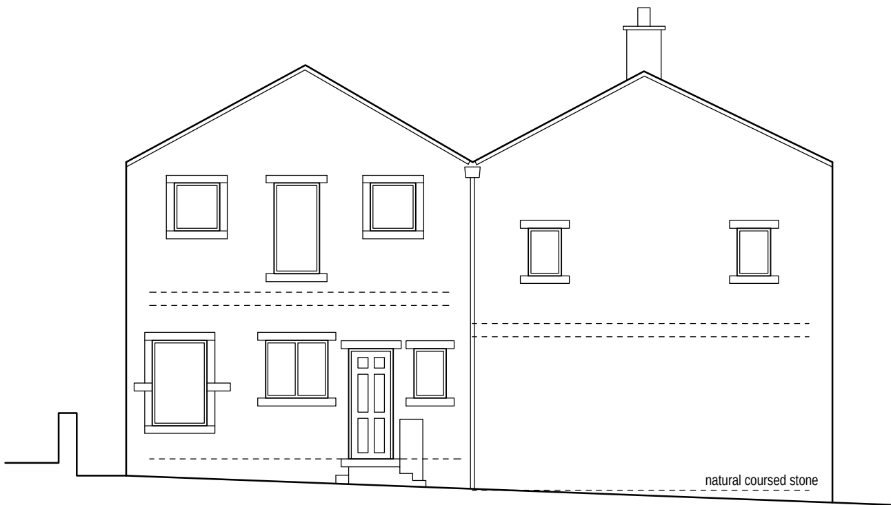
Existing front/south facing elevation (1:100)
