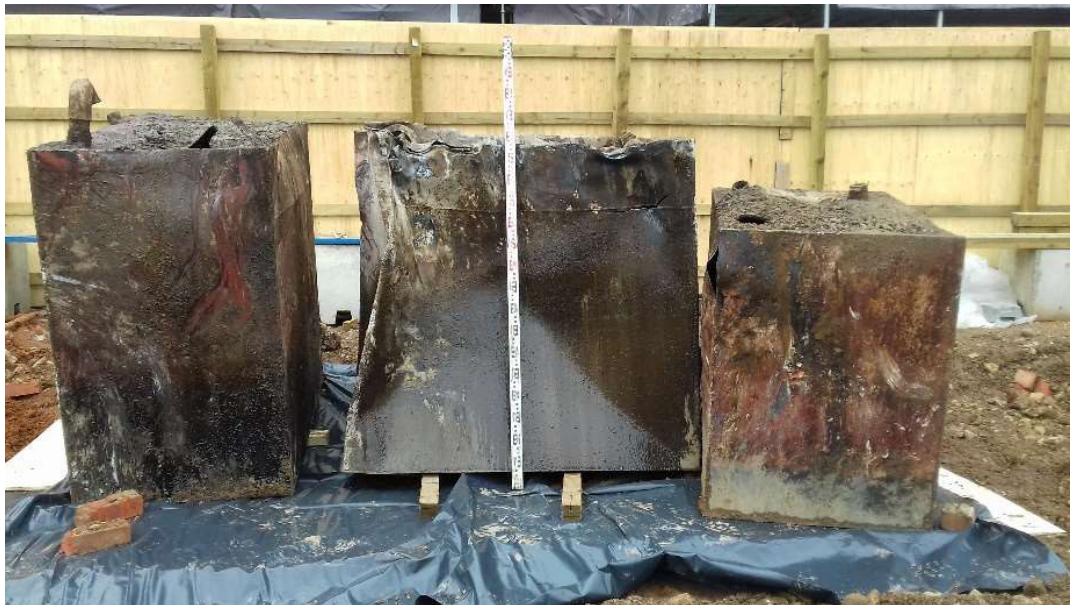
Figure F. Image of ASTs being inspected after a building demolition.
