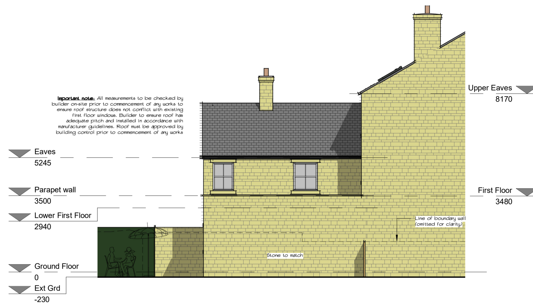
Side Elevation (West Facing) 1 : 100
