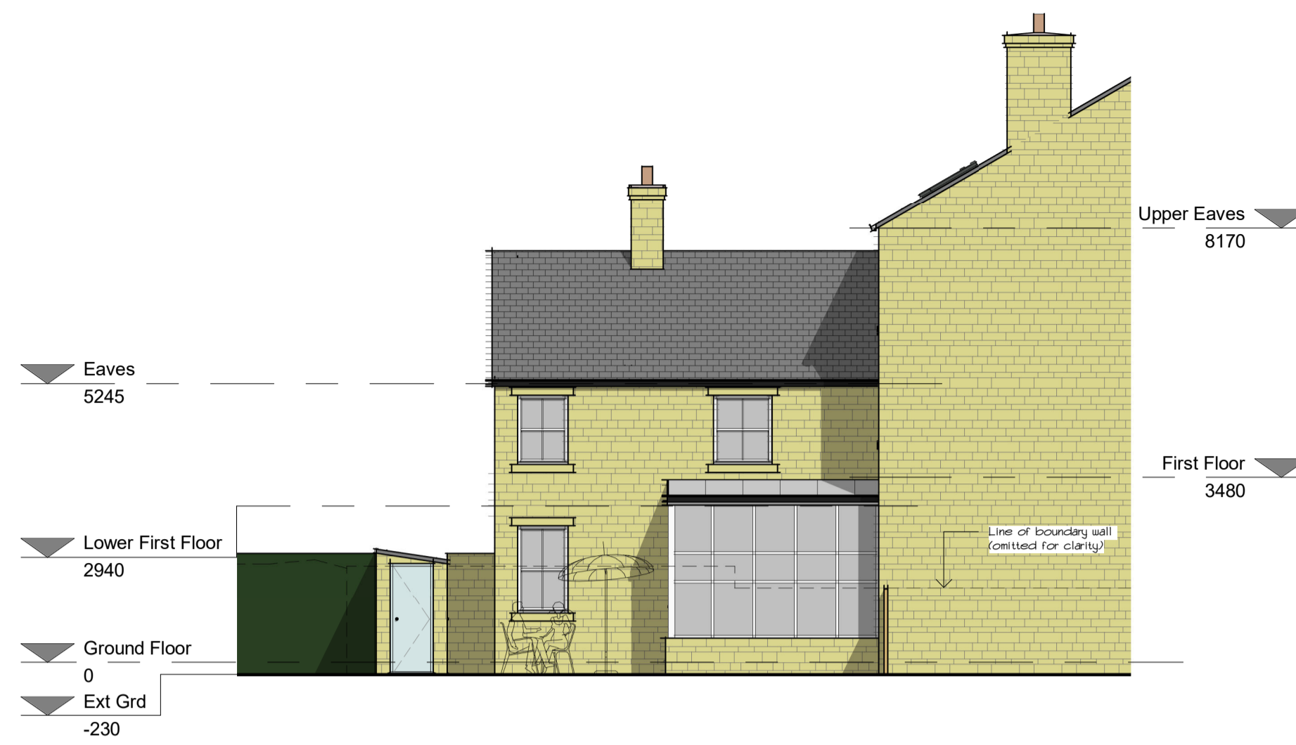
Side Elevation (West Facing) 1 : 100
