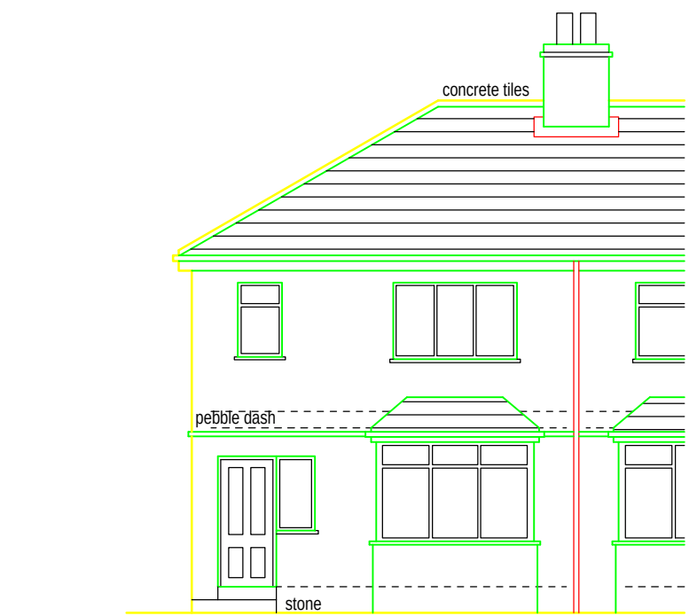
Existing front/north west facing elevation (1:100)
