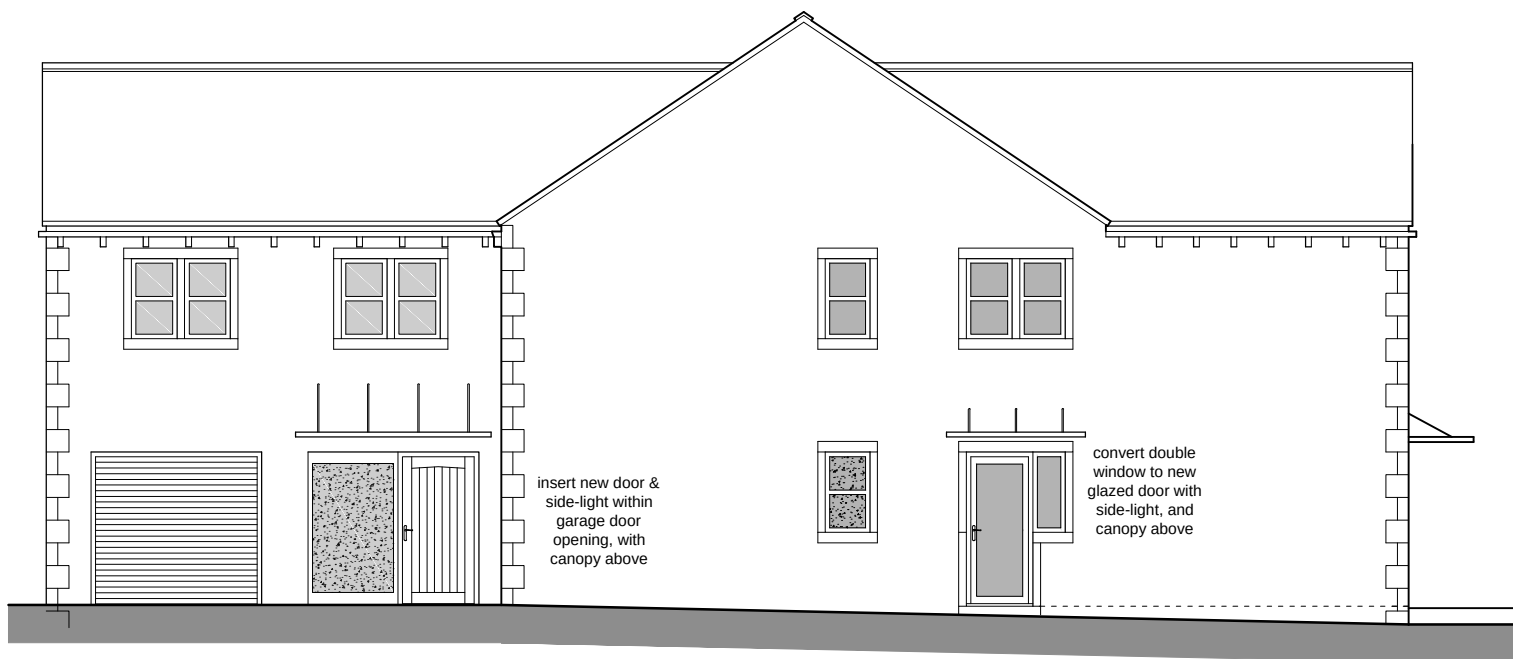
SOUTH WEST ELEVATION 1/100
