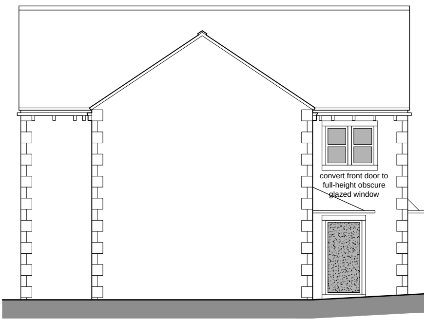
NORTH WEST ELEVATION 1/100
