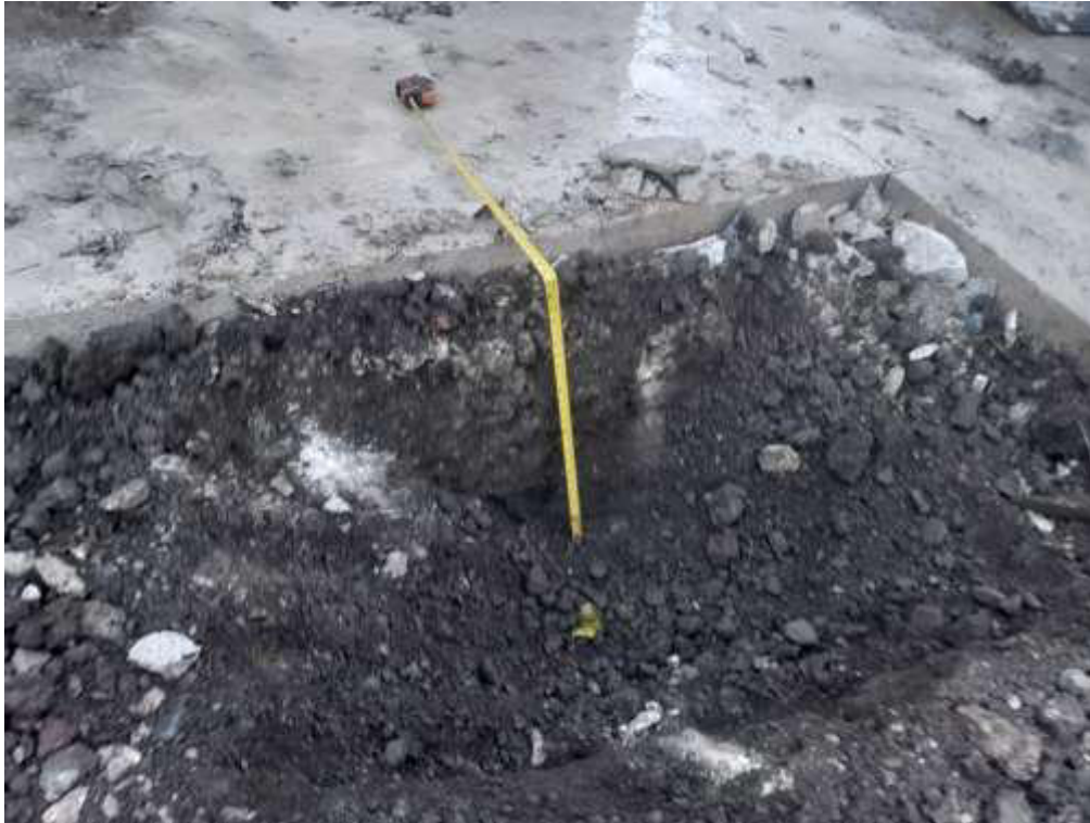
Plate 1: Picture of completed trial Pit
