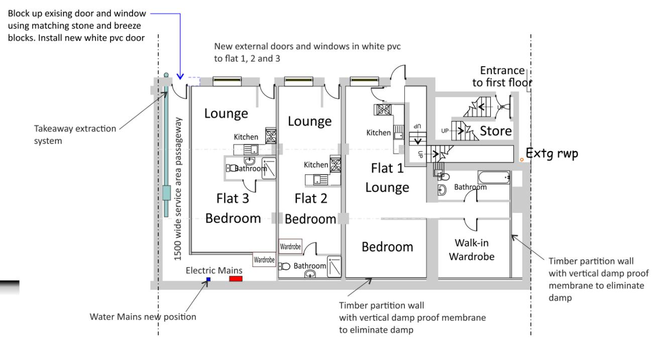
Proposed Basement Floor Plan Scale 1:200
