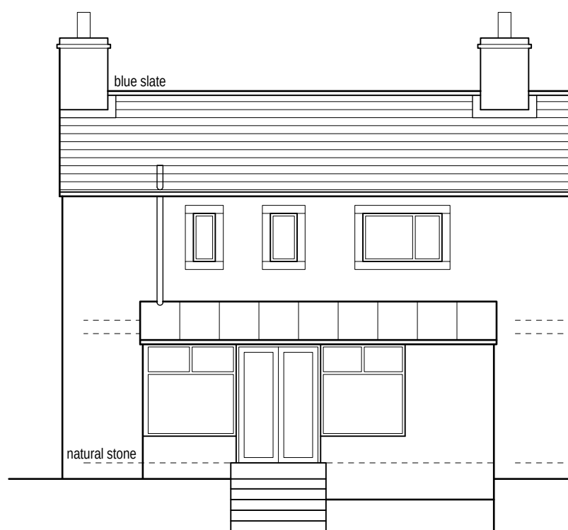
Existing rear/south facing elevation (1:100)
