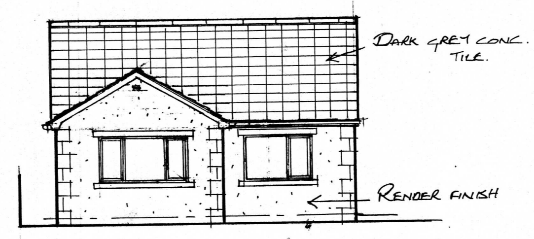
EAST ELEVATION (TO FIELD HEAD LN.)
