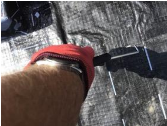
Plot 11 hand welded joint being pick tested
