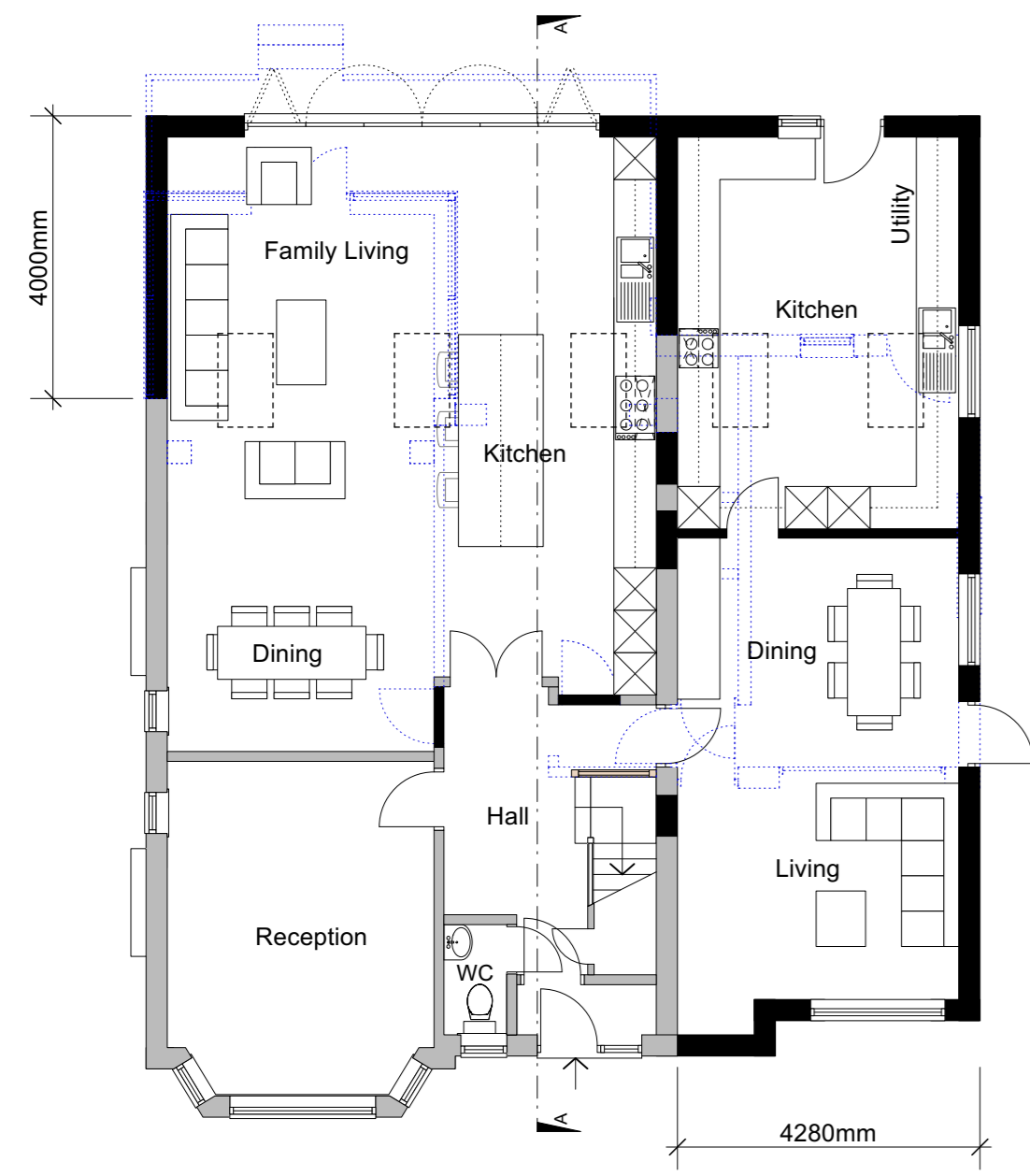
Ground Floor Plan As Proposed Scale 1:100 0m 1m 2m 3m 4m 5m
