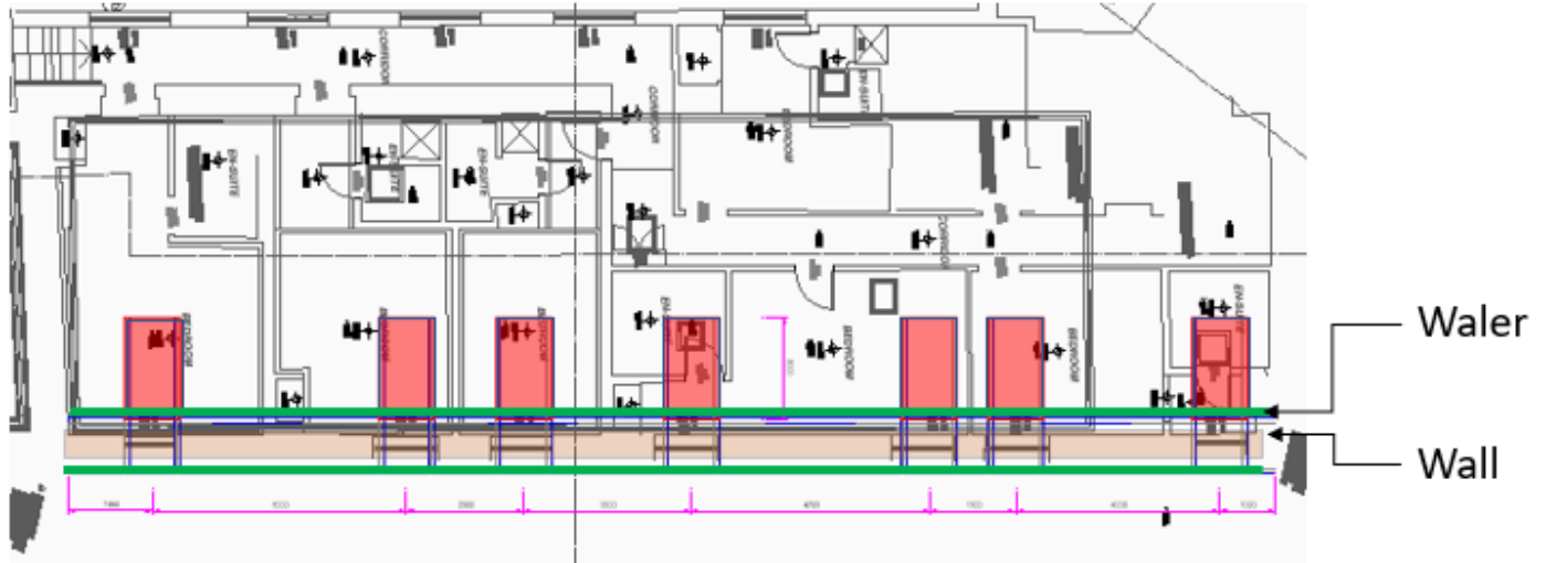
Figure 3: Plan View for Facade Retention - Option 2
