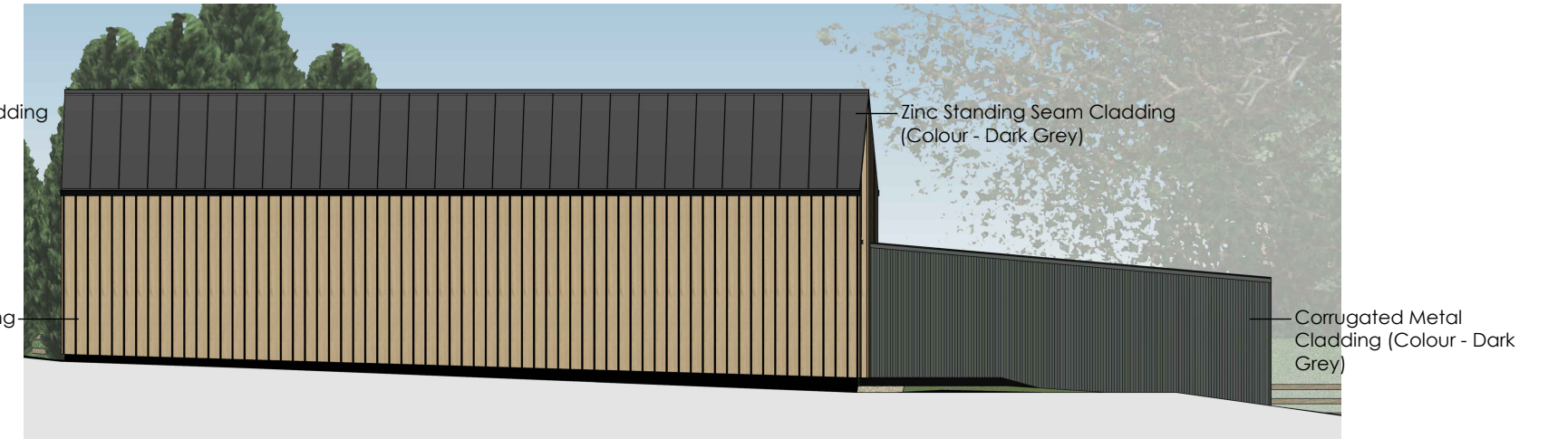
SOUTH WEST ELEVATION
