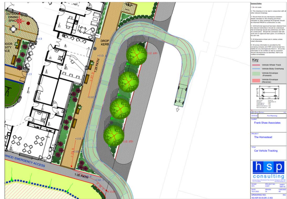
Figure 5: Car Vehicle Tracking
