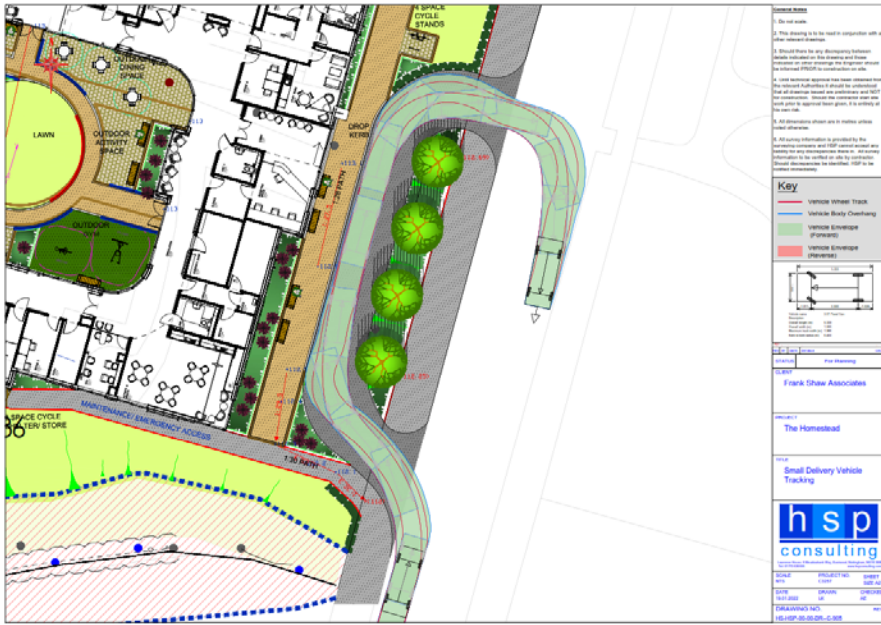
Figure 8: Small Delivery Vehicle Tracking
