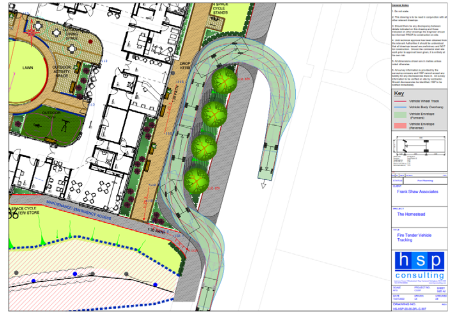
Figure 9: Fire Appliance Vehicle Tracking
