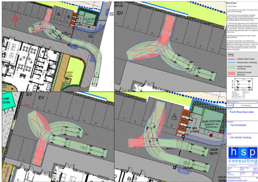
Figure 6: Car Vehicle Tracking
