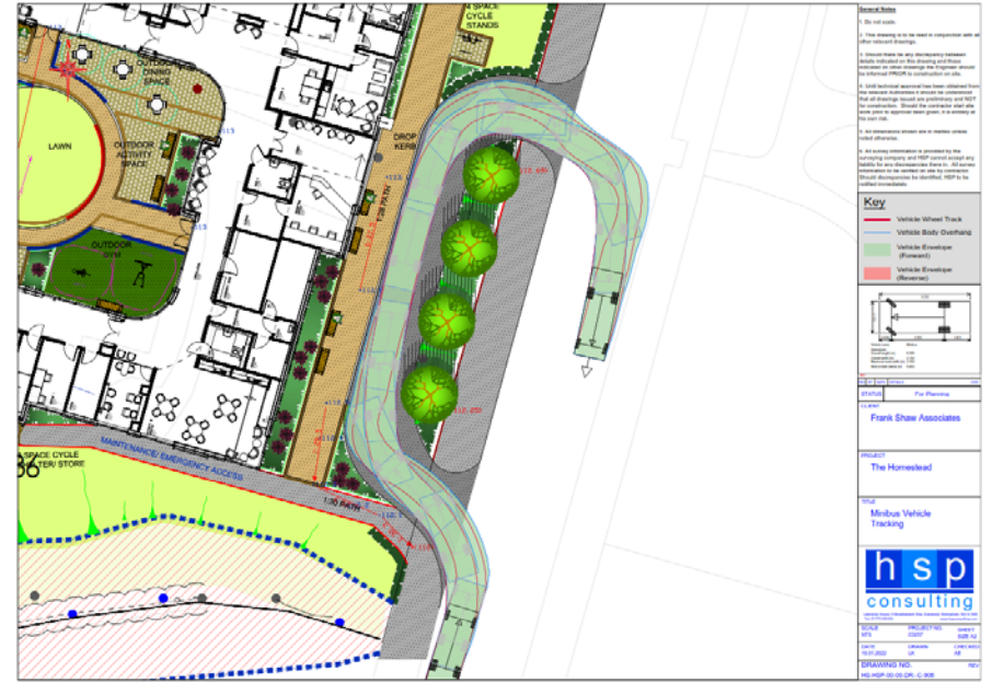
Figure 7: Minibus Vehicle Tracking
