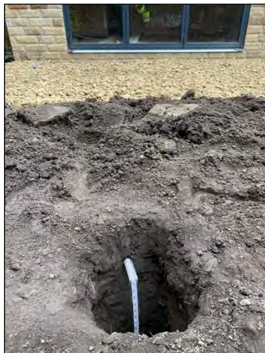
Garden area of house plots 11 and 13 showing the 600mm depth of topsoil in the excavated trial pits.
