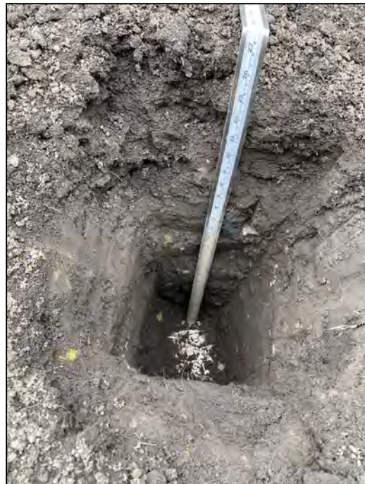
Trial Pits outside House Plot No 9 confirming 600mm of topsoil
