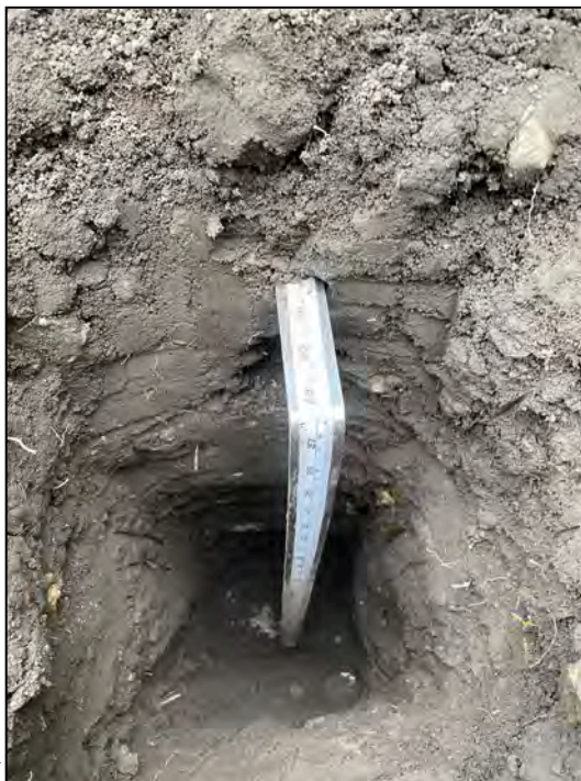
Garden area of house plots 11 and 13 showing the 600mm depth of topsoil in the excavated trial pits.
