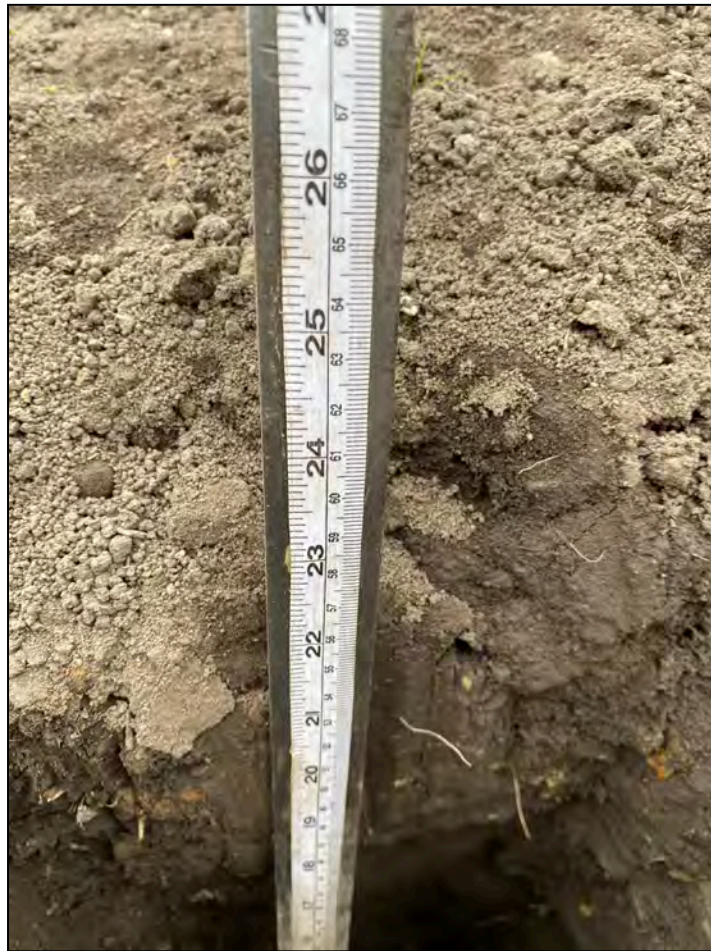
Close up of measuring pole in TP indicating topsoil depth greater than 600mm
