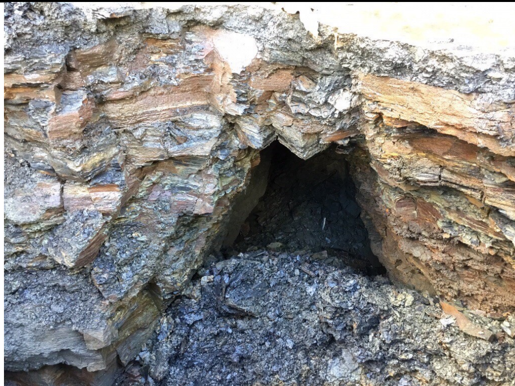
Photo 7: Workings identified at TP07. Extend off-site beneath no.52.
