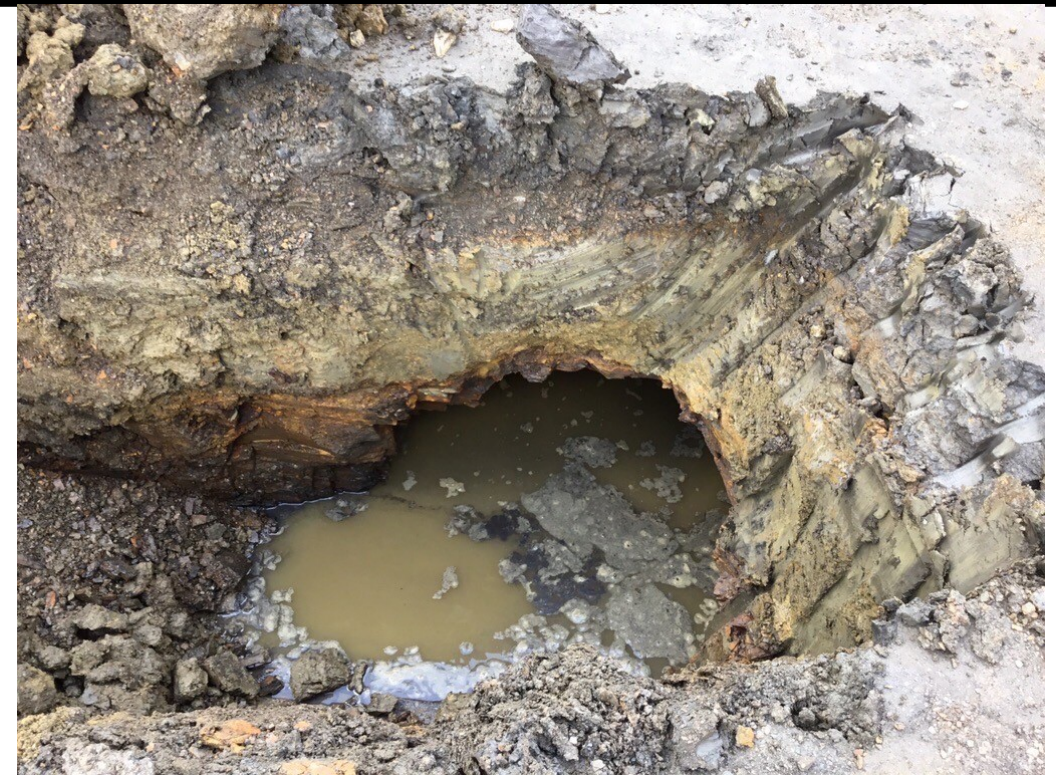
Photo 8: Coal workings identified at TP09.
