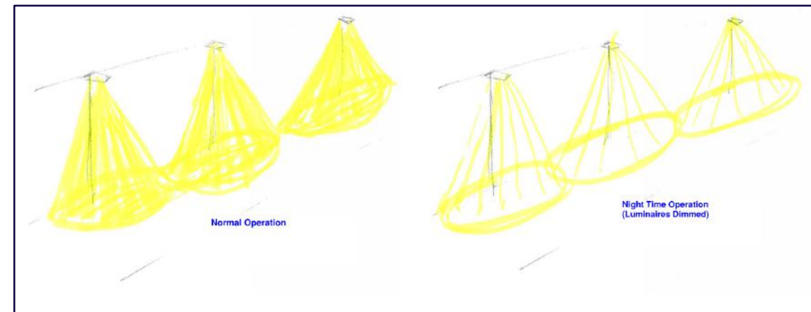
Figure 5-3 Alternatively dimming luminaires overnight.
