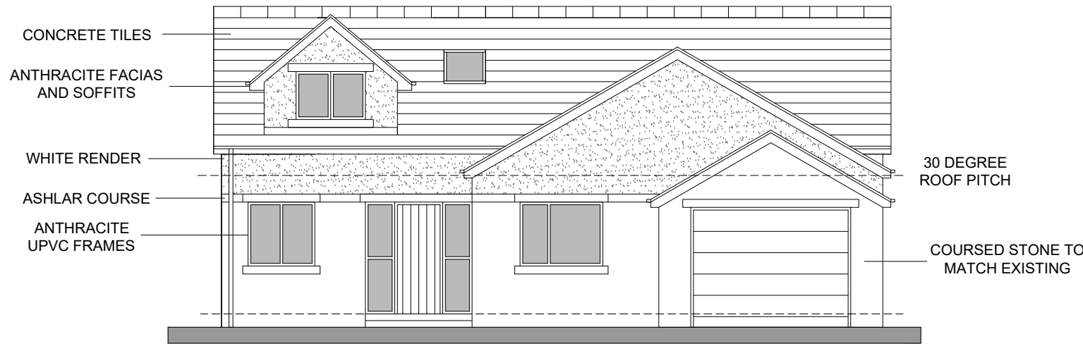
NORTH WEST ELEVATION
