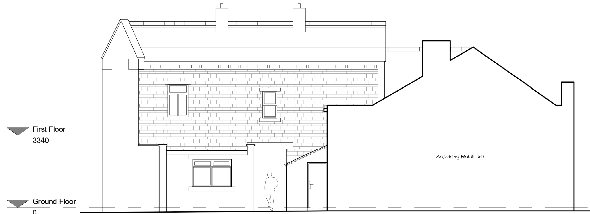
Side Elevation (North Facing) 1 : 100
