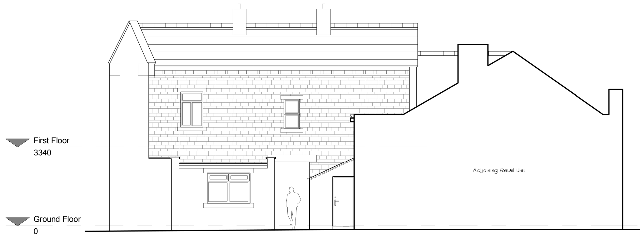
Side Elevation (North Facing) 1 : 100
