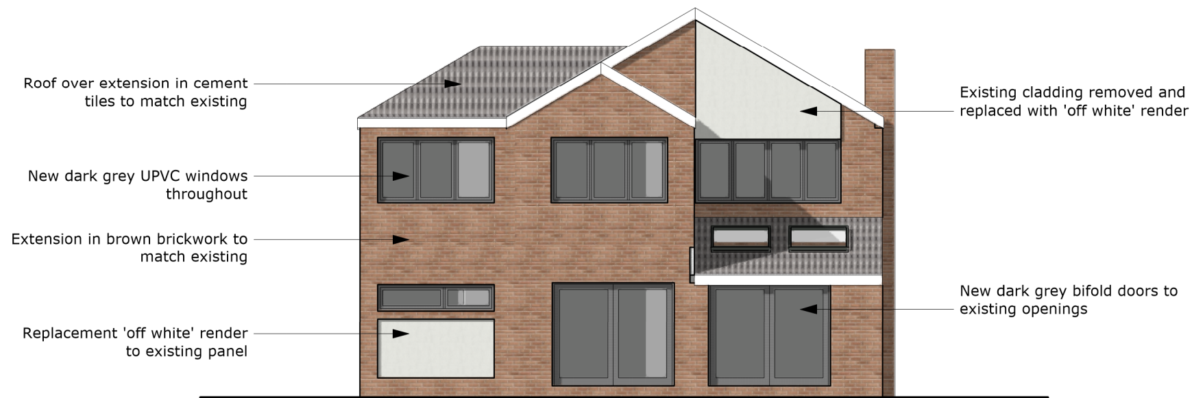
2 Proposed Rear Elevation Scale: 1:100
