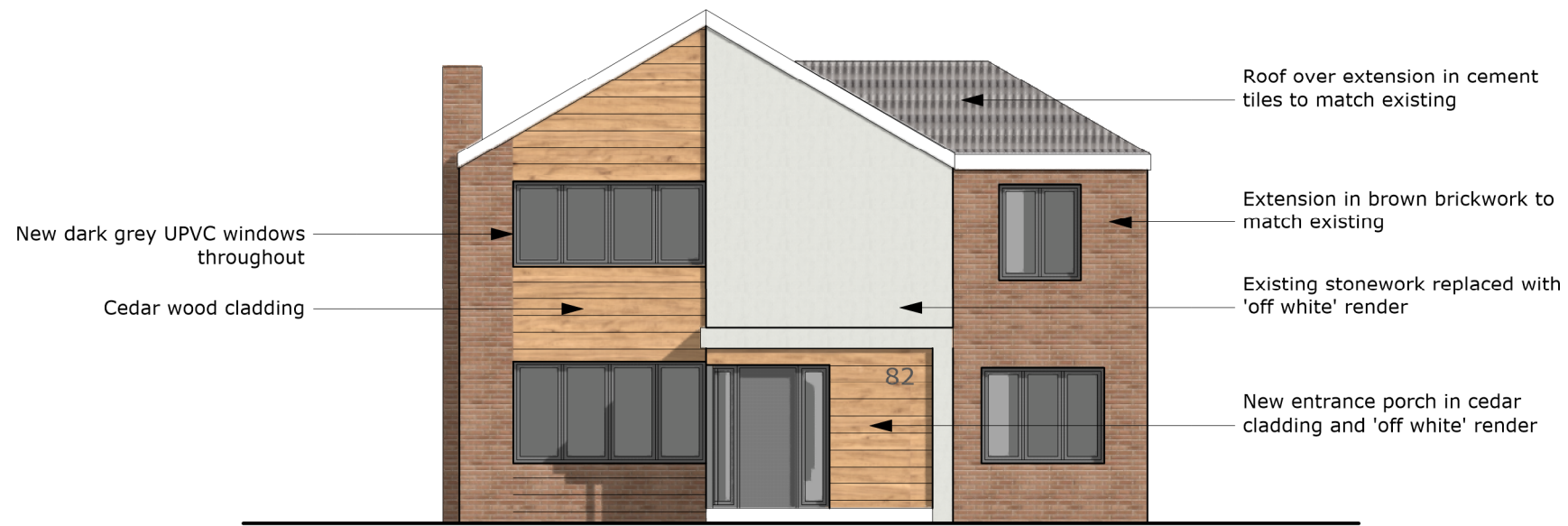
1 Proposed Front Elevation Scale: 1:100
