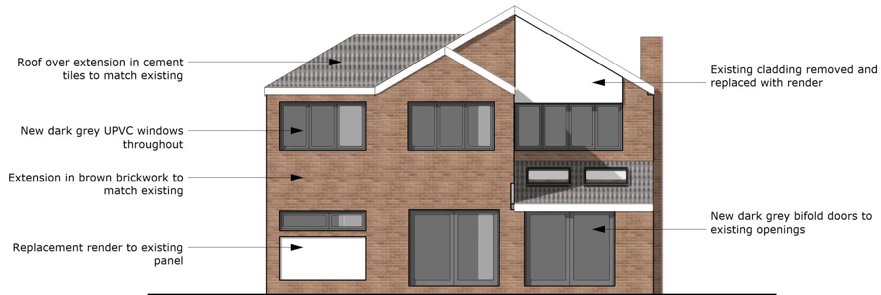
2 Proposed Rear Elevation Scale: 1:100
