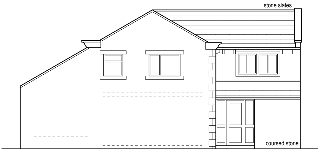
Existing side elevation (1:100)
