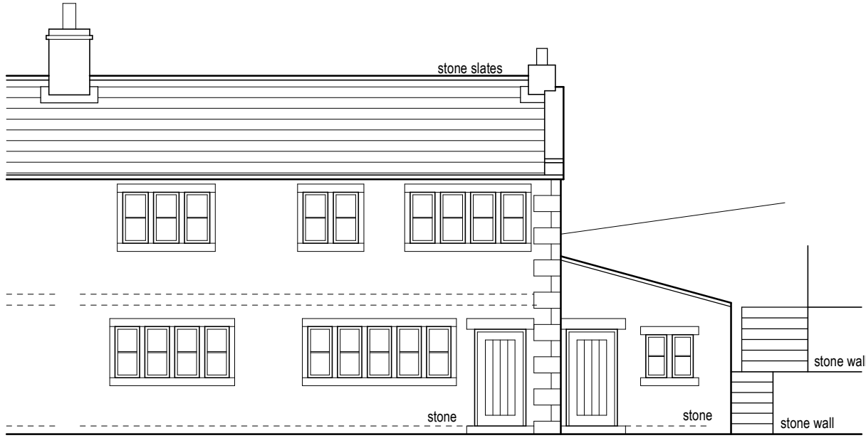
Existing front elevation (1:100)
