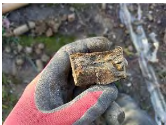
Photo 5: Showing the stiff friable sandy clay recovered at the base of WS01.
