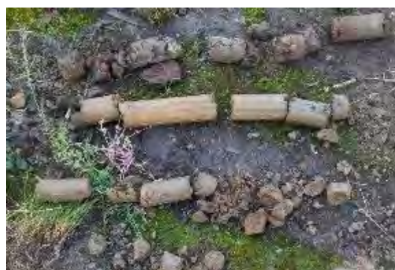
Photo 6: Showing recovered soils from ground level to 3m in WS04.
