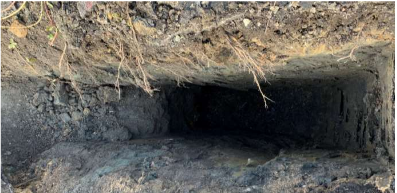
Photo 4: TP4 at a maximum depth of 3.00mbgl.
