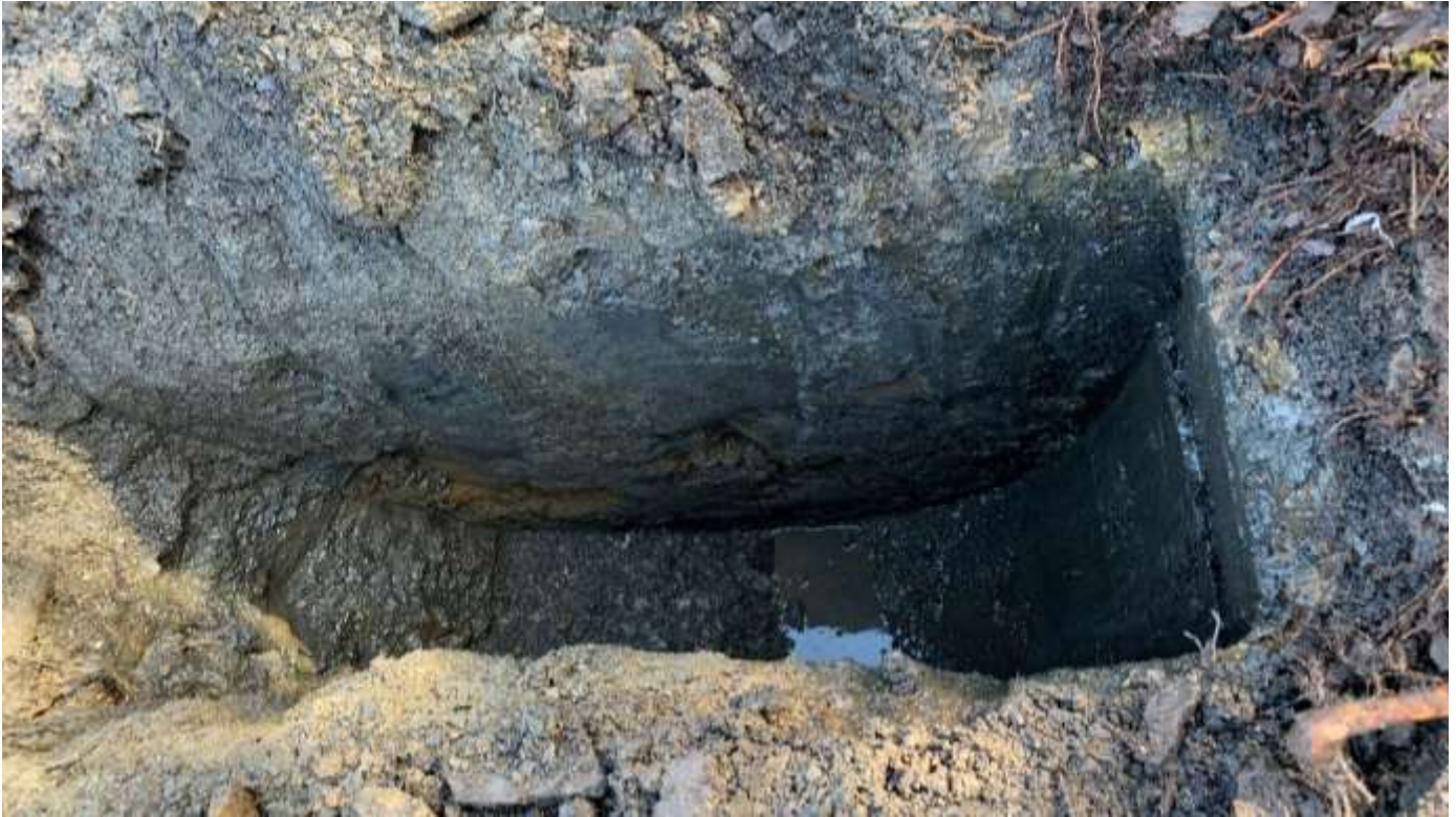
Photo 3: TP3 at a maximum depth of 3.00mbgl
