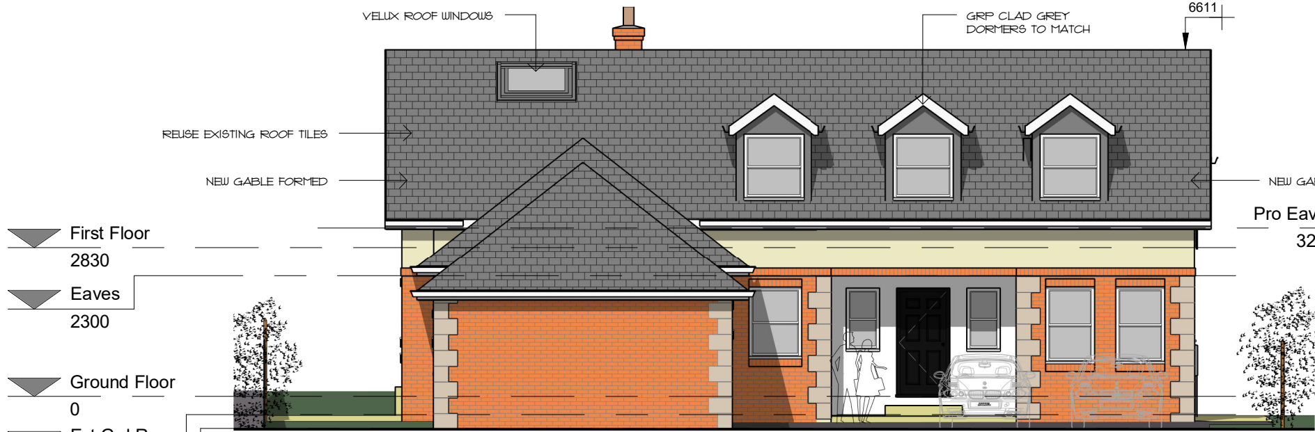
Front Elevation (East Facing) 1 : 100
