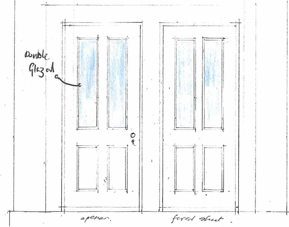
REAR ENTRANCE REOPENED. (Existing masonry retained)
