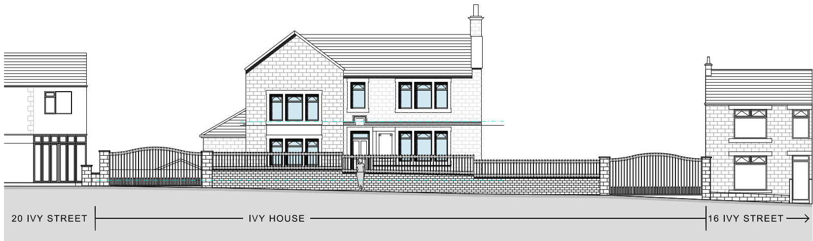
EXISTING STREET SCENE (BOUNDARY TREATMENT) ELEVATION
