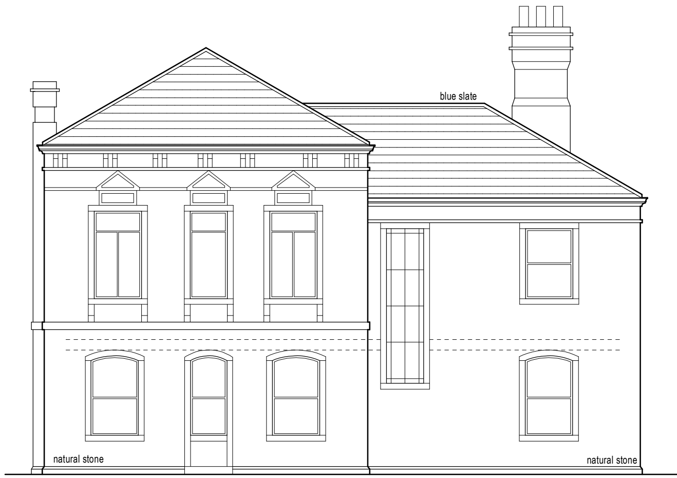
Existing rear elevation (1:100)
