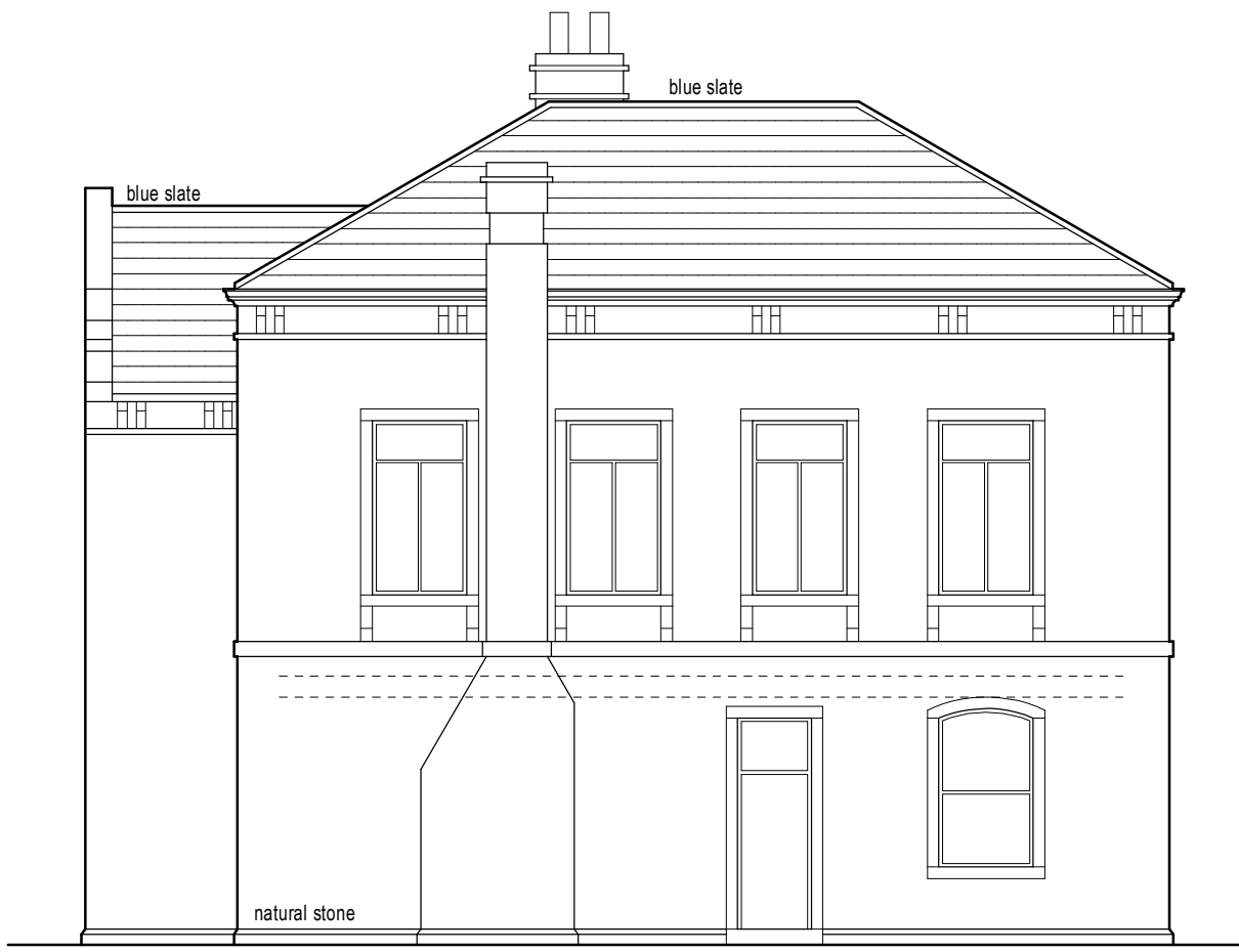
Existing side elevation (1:100)
