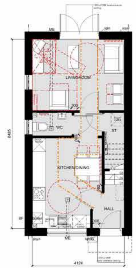
Ground Floor Plan Area to blockwork - 35.6m 2 (384ft 2 ) Area to plasterboard - 35.0m 2 (377ft 2 )
