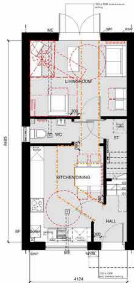
Ground Floor Plan Area to blockwork - 35.6m 2 (384ft 2 ) Area to plasterboard - 35.0m 2 (377ft 2 )
