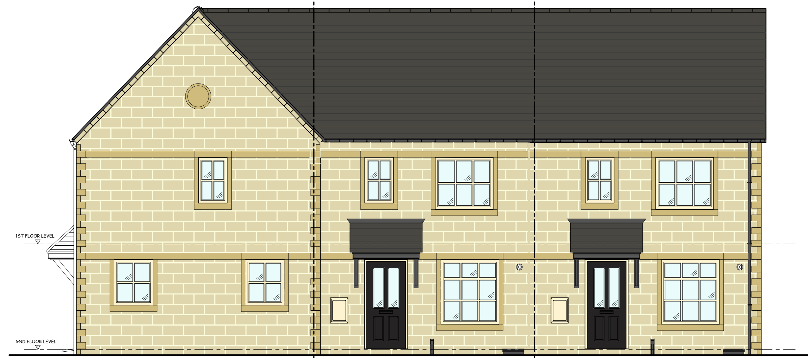
PROPOSED FRONT ELEVATION (1/50 SCALE)
