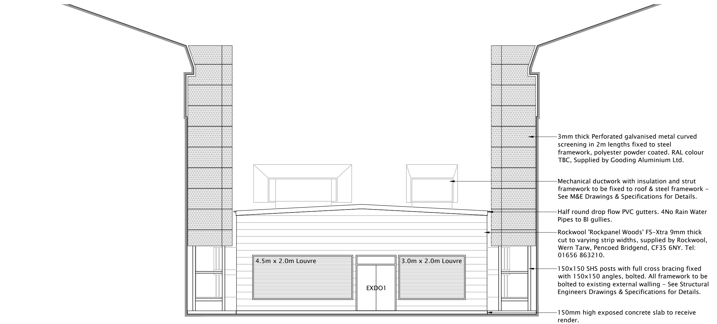
Elevation A as Proposed Scale 1:100
